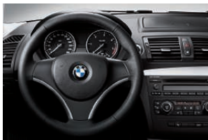
□ Sports leather steering wheel (diameter 369 mm) with thumbrests (in conjunction with gearshift paddles on the steering wheel without thumbrests), chrome clasp, three spokes (standard with 130i and 123d).
