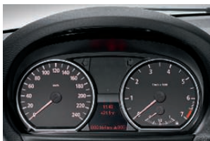
■ Instrument panel with analogue instruments and red backlighting: speedometer, LC display for mileage counter, trip counter and on-board computer, plus tachometer with integrated fuel gauge.
