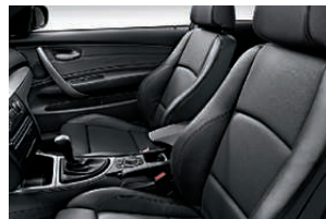
□ Sport seats for driver and front passenger (shown here with optionally available Boston leather upholstery in Black), with infinitely variable electric backrest width adjustment for optimum lateral support, plus manual adjustment of fore-and-aft position, seat height, backrest angle, seat angle and thigh support.
