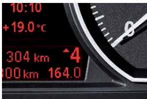
■ Optimum Shift Indicator shows when switching to another gear would be more fuel-efficient. The system recommends when to switch to a higher or lower gear, as appropriate to your driving style. For example, when accelerating it signals whether to carry on accelerating in a higher gear, thereby saving fuel (for vehicles with six-speed manual transmission).
