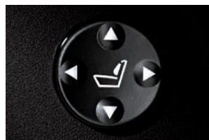
□ Lumbar support for driver and front passenger, electrically adjustable in height and length, for an ergonomically perfect seat position and support of the back muscles.
