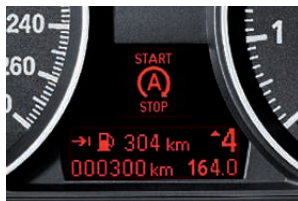
■ Auto Start/Stop display (for all four-cylinder models in conjunction with six-speed manual transmission) appears on the Info Display and indicates when the engine has been switched off by the Auto Start/Stop function (e.g. at traffic lights or in a jam). The signal disappears when the engine is automatically restarted.
