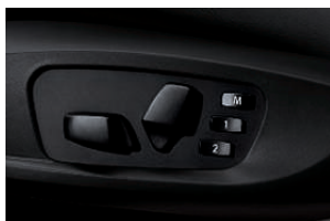
□ Seat adjustment for driver and front passenger with electric seat height and backrest adjustment, as well as back/forwards and seat angle adjustment, with memory function for driver's seat and exterior mirrors (including automatic parking function). Two personalised positions can be stored for the settings of the driver's seat and the exterior mirrors.
