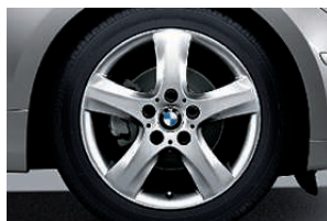
□ 17" light-alloy wheels star-spoke 142 with mixed runflat tyres, front 7 J x 17 with 205/50 R 17 tyres, rear 7.5 J x 17 with 225/45 R 17 tyres.
