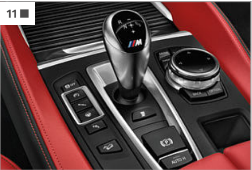
[ 11 ] The eight-speed M Steptronic transmission with DRIVELOGIC offers a variety of shifting options: from extremely dynamic, to comfortable, to fuel-saving.
