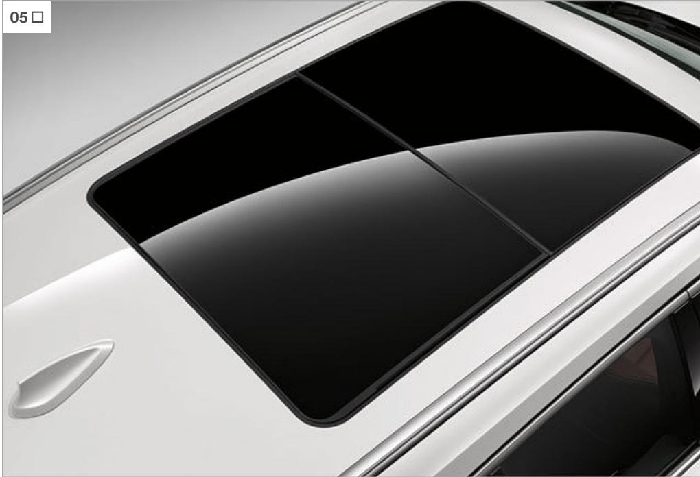
[ 03 ] Fog lights in the front apron provide better visibility and increase safety. [ 05 ] The panoramic glass sunroof has an automatic integral wind deflector, sun protection glass, independently sliding headliner panel and a comfort opening function via the car's remote key.
