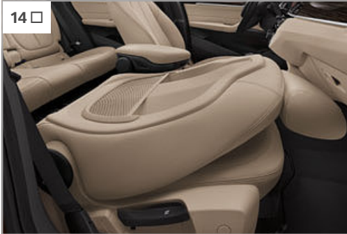
[ 11 ] The 40:20:40 split-folding rear seat bench with backrest manually adjustable three ways makes loading even easier, and the vehicle even more versatile.
