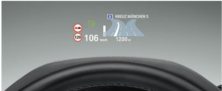
□ 610 Head-up Display , full colour, projects relevant driving information into the driver's field of vision thereby allowing the driver to always remain focused on the road ahead. Head-up Display shows information such as current speed, navigation directions, Speed Limit Info (if optionally fitted) including no-overtaking indicator, along with Check Control messages and infotainment information. 1
