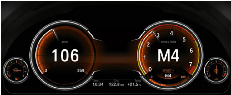
□ 6WB Multi-functional instrument panel , with Black panel technology and 10.25" display, provides an impressive visualisation of the driving experience. Three different modes and their specific characteristics – each of which have their own colour scheme and graphic style – can be shown in the display: Comfort, ECO PRO and Sport modes.
