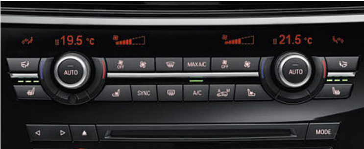
❑ 4NB Air conditioning, automatic with four-zone control (shown above), same features as two-zone automatic air conditioning, with additional air vents in the B pillars and separate controls for rear seat passengers. ■ Air conditioning, automatic with two-zone control features separate air volume and temperature controls for the driver and front passenger. Includes microfilter, fogging sensor, automatic air recirculation (AAR), as well as stationary cooling and residual heat functions.
