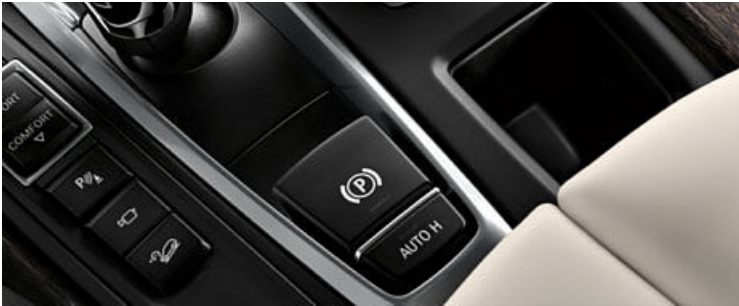
■ Parking brake with auto-hold function allows the brake to be applied and released via a button on the centre console. Auto-hold assists the driver in stop-start traffic, or during hill starts by preventing the car from rolling forwards or backwards when at a standstill.
