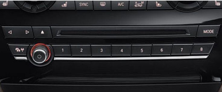
■ Favorite buttons - eight control buttons, positioned in the centre console, enable you to save and access frequently used items such as radio stations, telephone numbers and navigation destinations.
