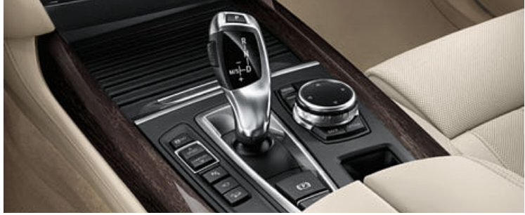
■ Eight-speed automatic transmission with Steptronic makes changing gears and driving significantly more convenient, thanks to fast engine speed transitions and shorter shift times. It unites outstanding comfort with palpable dynamics and increased fuel-efficiency. 2
