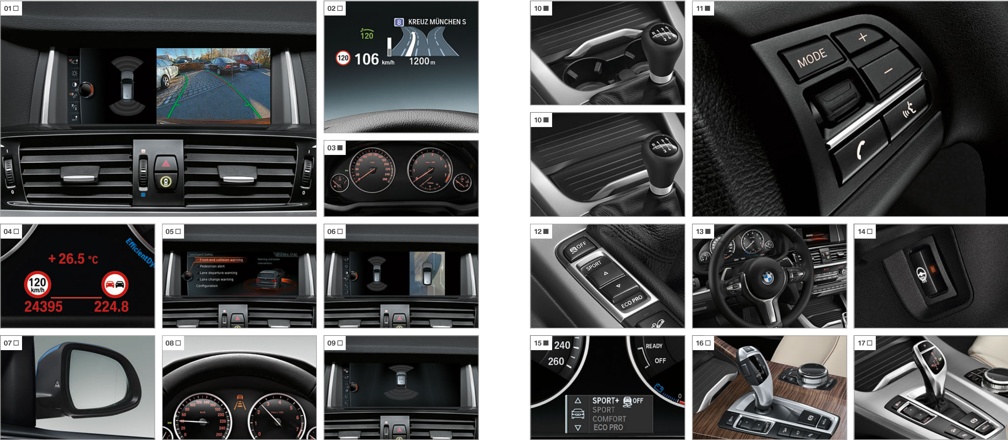
[ 01 ] Reversing Assist camera shows the area behind the car on the Control Display. Interactive track lines provide assistance when manoeuvring or parking. [ 02 ] Head-up Display transmits driving-related information directly into the driver's line of vision. 1 [ 03 ] The instrument cluster features four analogue dials including a speedometer, rev counter and coolant temperature display, as well as a 2.7" Info Display. [ 04 ] Speed limit display including no-overtaking indicator provides information on speed limits as well as no-overtaking zones. [ 05 ] Driving Assistant combines Lane Departure Warning and Approach Warning systems. [ 06 ] Surround-view is a visual parking aid. The immediate 360 degree environment is shown on the Control Display via cameras on the vehicle. [ 07 ] Lane Change Warning detects other vehicles when changing lanes and warns the driver through vibration in the steering wheel and a triangular warning symbol on the wing mirrors. [ 08 ] Driving Assistant Plus includes Approach and Lane Departure Warning and Active Cruise Control with Stop&Go function. [ 09 ] Park Assist makes parallel parking easier. It steers while the driver controls the accelerator and the brake.
