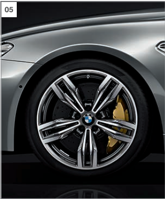
[ 05 ] 20" M light alloy Double-spoke style 433 M wheels with mixed tyres. Front: 9.5J x 20 with 265/35 ZR20 tyres. Rear: 10.5J x 20 with 295/30 ZR20 tyres.
