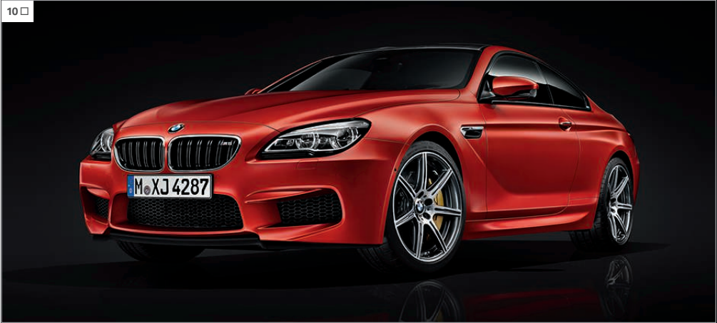
[ 09 ] For the ultimate adrenalin kick, the output of the M TwinPower Turbo eight-cylinder petrol engine has been increased from 560hp (412kW) to 575hp (423kW). This enhanced performance is achieved by raising the boost pressure in the upper rev range.
