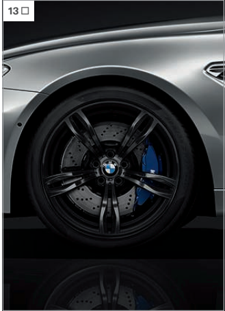
[ 10 ] 20" M light alloy Double-spoke 433 M wheels in Orbit Grey with mixed tyres. Front: 9.5J x 20 with 265/35 ZR20 tyres. Rear: 10.5J x 20 with 295/30 ZR20 tyres. (Standard with M6 Gran Coupé).
