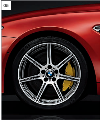
[ 05 ] 20" M light alloy Double-spoke style 601 M wheels with mixed tyres. Front: 9.5J x 20 with 265/35 ZR20 tyres. Rear: 10.5J x 20 with 295/30 ZR20 tyres (only available with Competition package).
