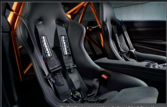
The Club Sport package combines the 6 point Schroth Racing Harnesses for ultimate stability, the Multi point steel roll cage in Acid Orange and a rear mounted fire extinguisher. Combined with the weight optimised CFRP bucket seats with high-grip, hardwearing Alcantara and leather upholstery, it ensures a heightened motor sport experience.
