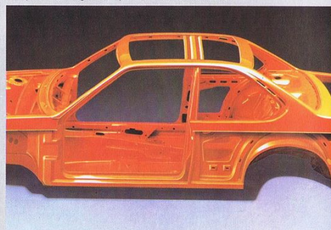
Passenger compartment protected by sturdy front bulkhead and shaft tunnel.
