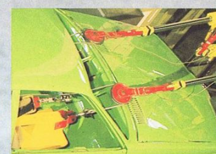
Seat belt anchor-point strength test.
