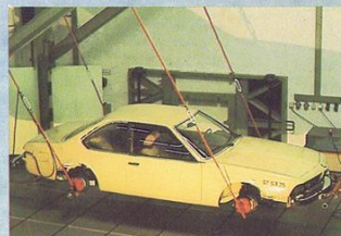
Bumper strength test.
