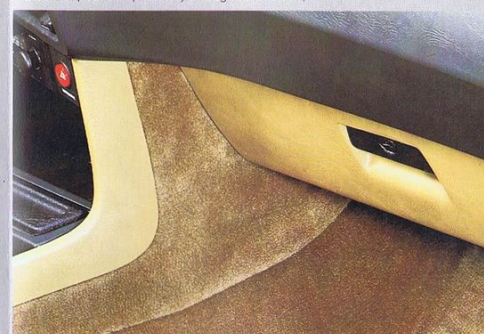
Safety padding extends from instrument panel down to knee area.
