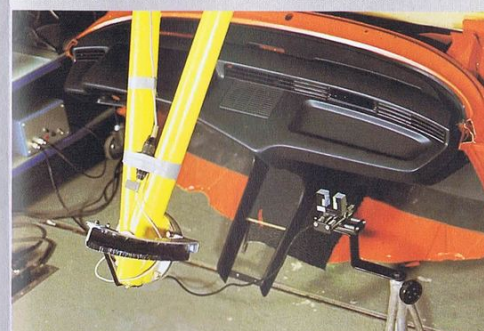
Pendulum impact test of energy absorbing instrument panel.
