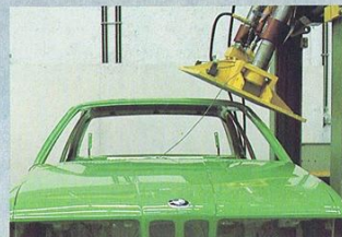
Roof strength test.
