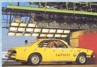
Head-on collision testing at 30 mph.
