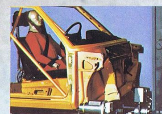
Seat belt system tested on sledge impacts.
