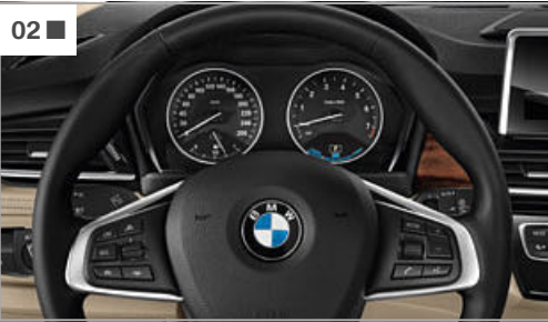
[ 01 ] The driver can choose from three electric drive modes by pressing the eDrive button: AUTO eDrive (standard), MAX eDrive or SAVE BATTERY.
